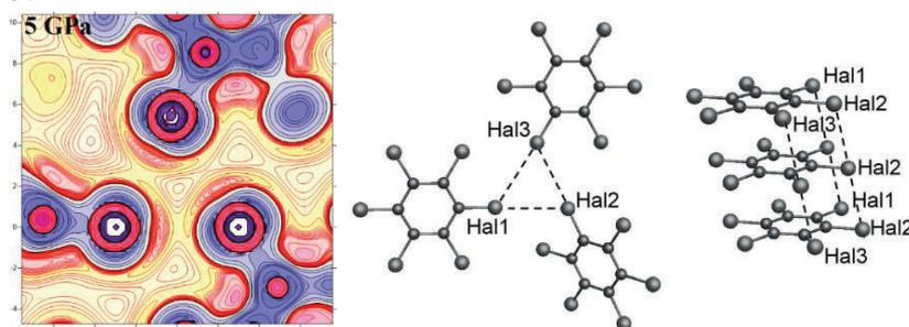
Figure 1: Quantum electronic pressure for Hal<sub>3</sub>-synthon in C<sub>6</sub>I<sub>6</sub> crystal
